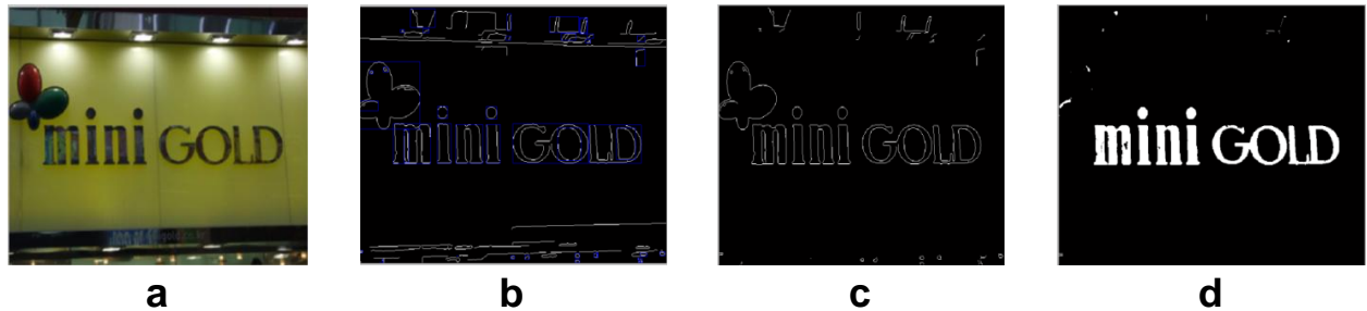
Figure 1. The proposed algorithm results from Level 1 (a) Original image; (b) Result image after connected component labeling; (c) Result image after text candidates selection; (d) Result image after text extraction - level 1.
